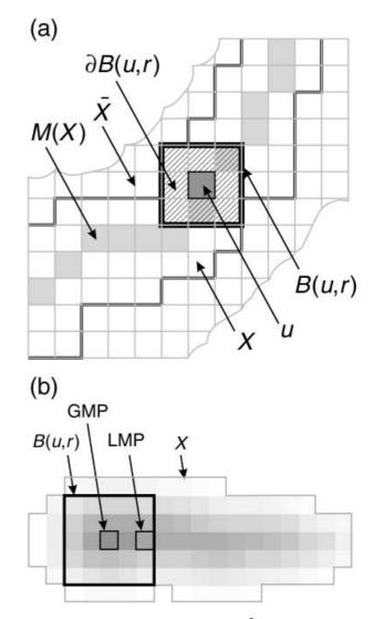
**Fig. 3.** (a) The illustration of definitions of *X*,  $\bar{X}$ , *u*, B(u,r),  $\partial B(u,r)$  and M(x). Detailed description in text. (b) Euclidean distance mapping (EDM) converted a binary image to a grey-scale image in which pixel value codes the Euclidean distance from each pixel within the object *X* to the nearest background  $\bar{X}$ . Description of GMP and LMP in text.
