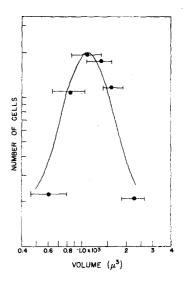
Fig. 3. Comparison of the shapes of the light scattering ( $\bullet$ ) and Coulter volume distributions (—) for a 6 to 8  $\mu$  diam fraction of Dow microspheres obtained with
