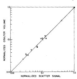
Fig. 2. Comparison of Coulter volume and scatter signal for various samples of plastic microspheres normalized to ragweed pollen: (x)—Dow latex spheres; (O)—3M Corporation carbonized plastic spheres; (E)—Dow latex spheres dyed black; and (D)—the same Dow latex spheres undyed.
