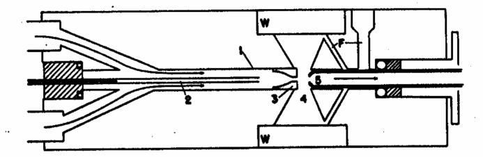
Fig. 2. The flow chamber (scale 4 times actual). W = window; F = flushing system for bubble removal; 1 = sheath flow; 2 = sample injection; 3 = nozzle; 4 = quiescent (viewing) region; and 5 = exit tube.
