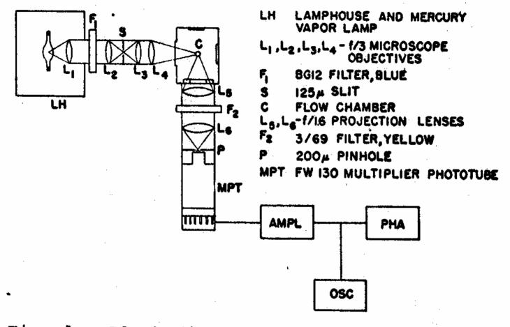
Fig. 1. Block diagram of fluorescent cell photometer.
